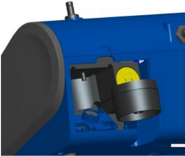
Figure 4-8: Remove 37-mm Filter Cassette
