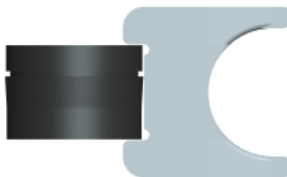
Figure 4-10: Replace Mesh in Filter Holder
