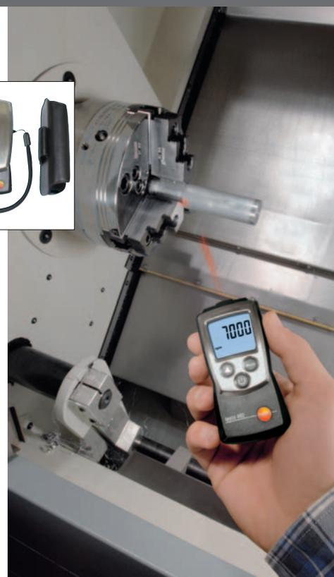
rpm measurement on shafts
