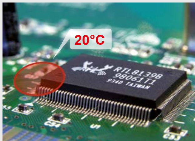
Spot size chosen too big which results in a measurement error
