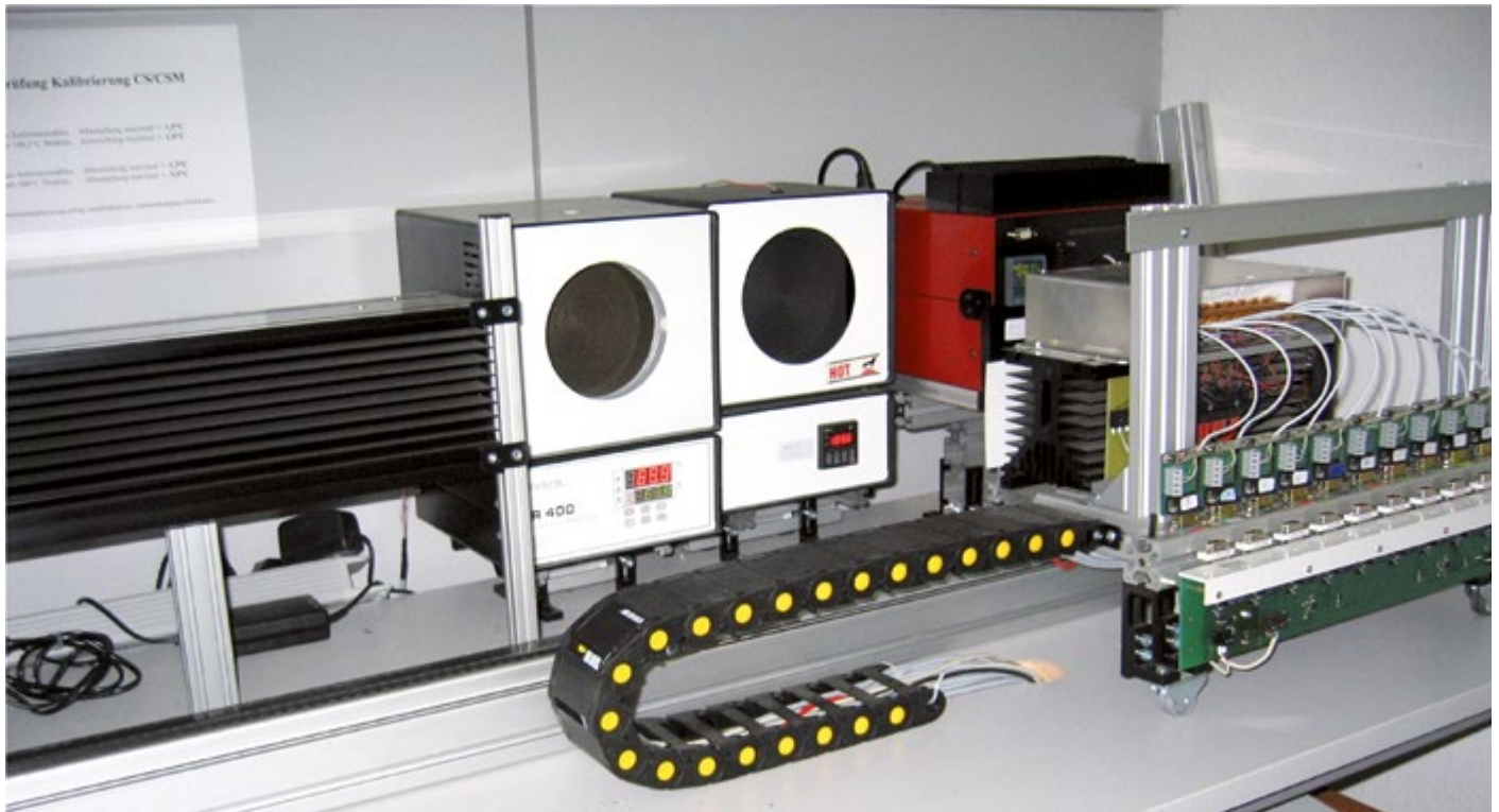
Automated calibration stations at Optris GmbH
