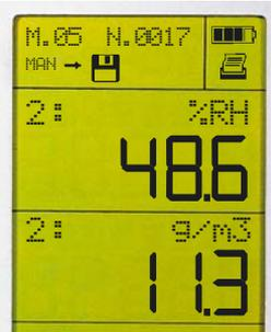
Automatic calculation of different humidity parameters in the instrument
