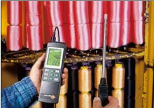
Measuring humidity at up to +180°C in drying systems
